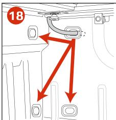
Route the front drain hoses from the end of the rail out through manufacturer avail - able bed plug. Simply remove these plugs or drill a 7/8" hole through the plastic. If you have a drop in plastic bedliner, simply run the drain tubes behind or under the liner.
