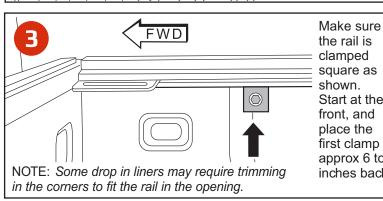
the rail is clamped Make sure the square as clamp is inserted shown. all the way up Start at the into the rail and front, and clamp teeth are place the alinged to rail first clamp slots to ensure approx 6 to 9 inches back. a secure grip.
