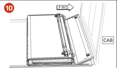
The small panel faces forward, toward the cab and folds down over the slotted rail brackets. The front panel must sit just inside the bulkhead rail with the seal resting on top of the bulkhead. Fold the panel down and align it so it is setting squarely on the rails and align the mounting holes with the slotted rail brackets.
