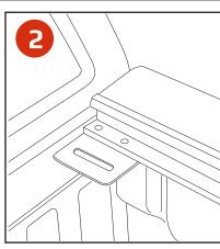
Close tailgate. Place BAKFlip rail on truck bed with silver bracket all the way forward and toward the center of bed as shown. Refer to enclosed Spacing & Shimming Sheet for more details. Rails should be completely level.
