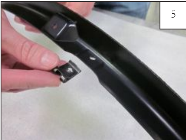
Verify presence of U-Clips on inner brackets.
