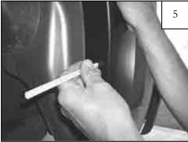
Holding flare in position on fender, use a grease pencil to mark five clip locations. See step 6.
