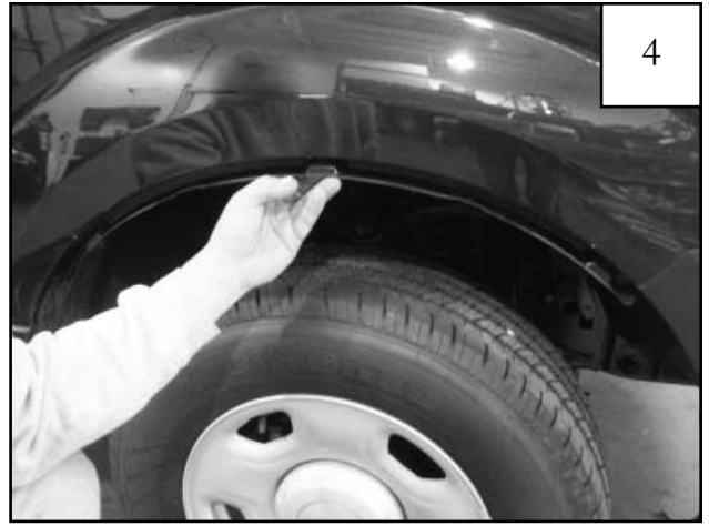
Line up the holes in the inner piece with the two uppermost factory holes and the speed clip. NOTE: Driver's side inner piece is marked with an "L" and passenger's side inner piece is marked with an "R".
