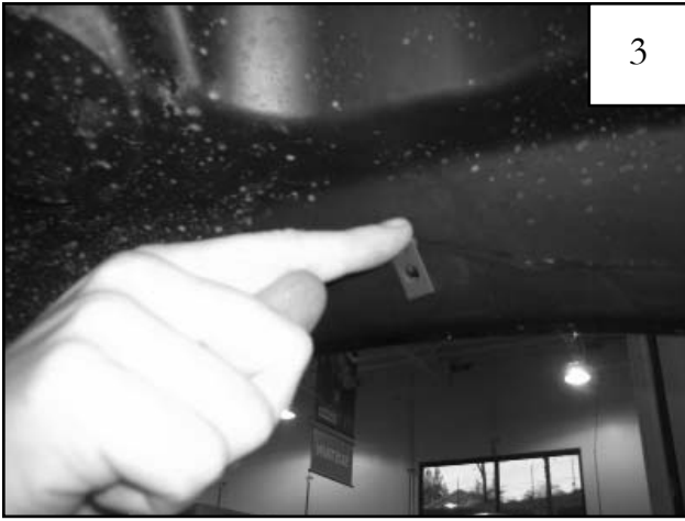
Place speed clip over existing factory hole.
