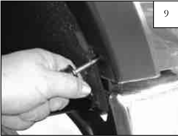
Still holding flare to fender, install tuftlocks using a Phillips screw driver. See step 10.
