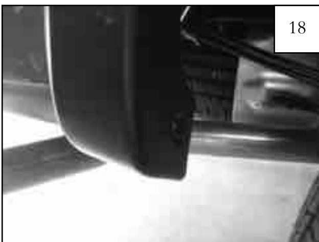
18 Install tuflock through hole in inside of rearward end of wheel well. See step 18.
