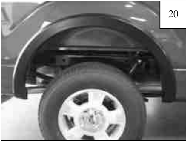
Completed rear flare installation.
