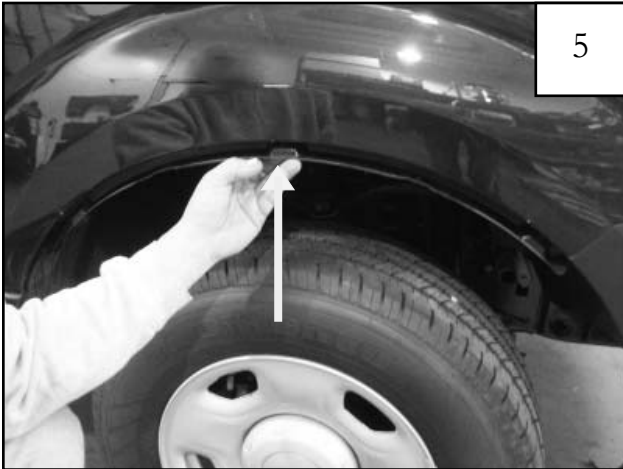
Using a Phillips screw driver, start a pan head screw through center hole in inner piece and through the speed clip over the fender wheel well lip.
