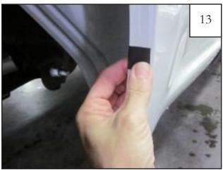
Wrap a Foam Tab (MT1-0034) around the wheel well sheet metal, centered over each of the upper four marks made in Step 12. Place a Mylar Tab (MT1-0014) at the mark made on the lower front of the wheel well.
