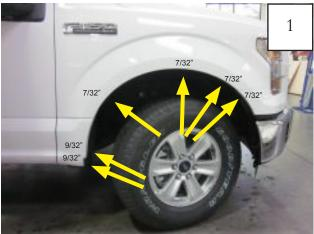
Remove four factory screws with a 7/32" socket wrench, (start from the second front). Remove two rear most factory screws with 9/32" socket wrench. Save screws for reinstallation.
