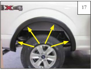
While holding flare to vehicle, start supplied screws (SW1-0058) through the four topmost mounting holes in flare and into the clips installed in Step 15.
