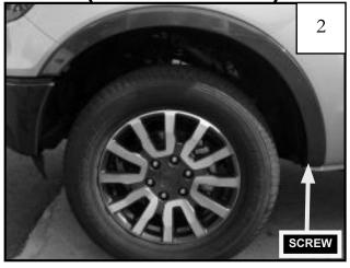
Remove (1) factory installed screw from the rear of the fender trim using a T-25 Torx driver. The screw will be re-used to install the front flare.
