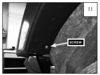
Install (1) truss screw (SW1-0050) through the front hole in the flare into the "S" spring clip using a #2 phillips screwdriver.
