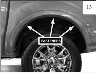
Remove (3) factory installed plastic fasteners from the driver side rear wheel well using a phillips screwdriver. Needle nose pliers may be needed to extract the fasteners.
