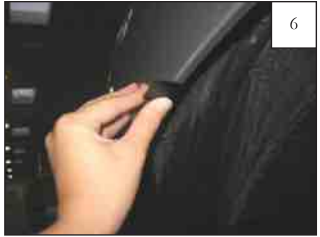
Remove flare from fender. Center a supplied Black Tab over each mark made in Step 4.
