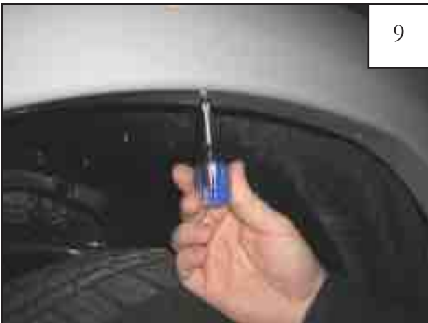
Replace flare on fender, aligning holes with holes in clips. Start three supplied Serrated-Flange Screws through three holes in flare and into "S" Clips installed in Step 7.
