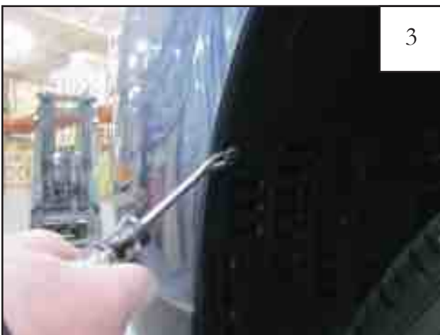
Using a pry tool, remove two plastic factory fasteners.
