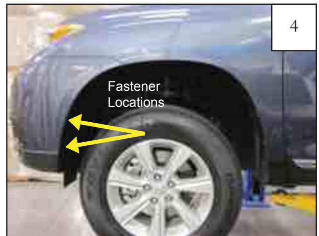
Factory fastener locations.
