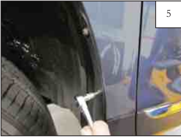
Using a 3mm Allen Wrench, remove two factory screws from rear of wheel well. Save for reinstallation.
