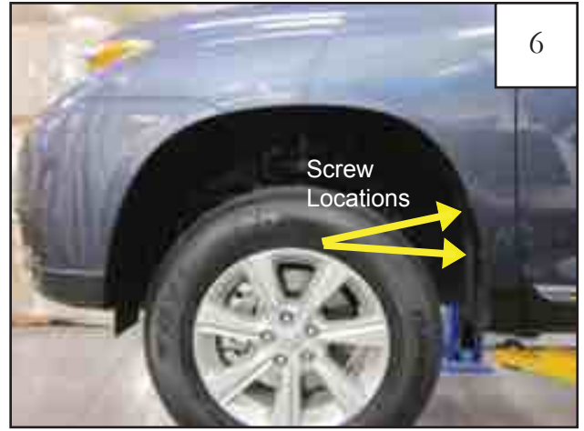
Two factory screw locations.
