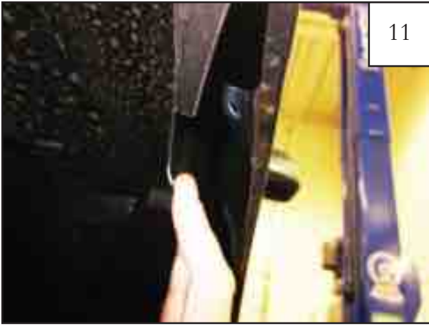
Install Tab (MT1-0017) over factory hole locations behind wheel well liner. Reference Step 8 for locations.
