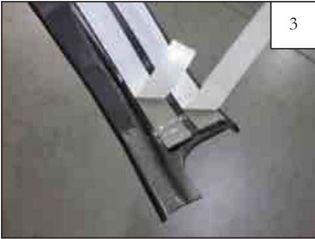
Start to peel white vinyl liner from tape at bottom of Inner Door Piece, folding tabs toward the outer curvature of the part and ensuring that inner liner is behind the outer liner.
