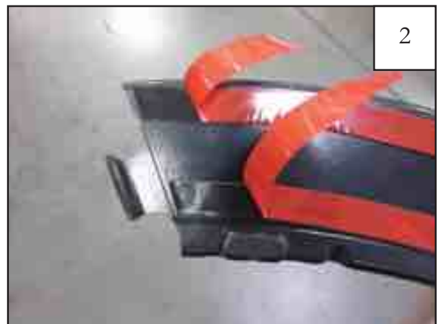
Start to peel red vinyl liner from tape at top of Inner Door Piece, folding tabs toward the outer curvature of the part and ensuring that inner liner is behind the outer liner.
