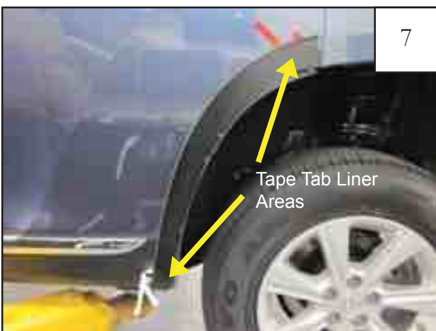
Ensure that tape tabs are accessible, top and bottom.
