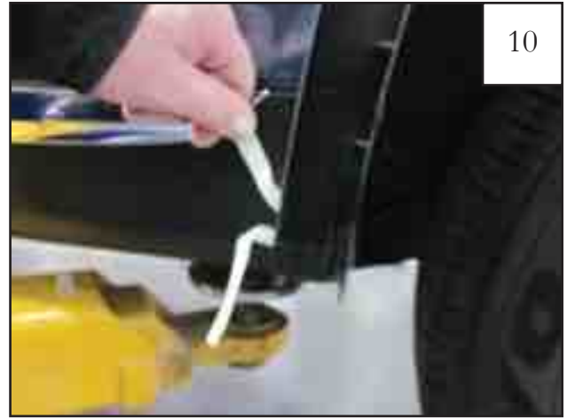
Pull white tape liner at the top (tape closest to the edge of the door).
