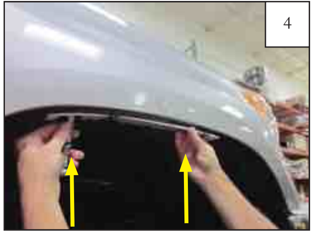
Using two supplied 20mm Hex Screws (SW1-0036), attach bracket to factory holes with a 10mm socket.
