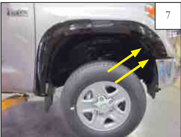
Start two supplied 20mm Hex Screws through forward most holes in flare and into factory hole locations.
