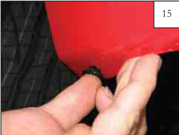
Note: If the lower rear wheel well does not contain a plastic grommet, insert a supplied one into the factory hole as shown.
