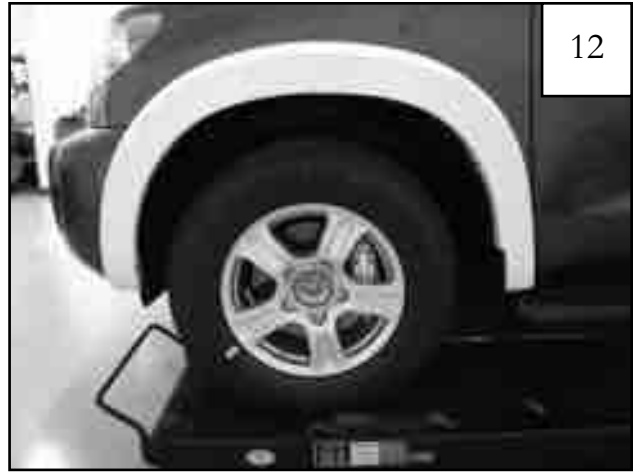
Starting at rearmost fastener, apply pressure towards vehicle at each fastening point as you tighten all screws (working your way to the front).
