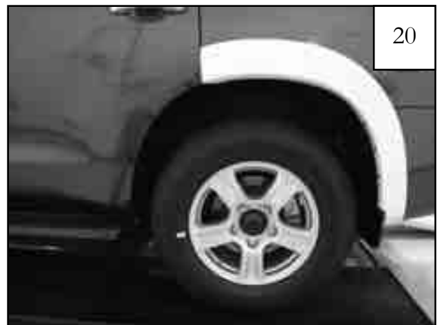
20 Starting at rearmost fastener, apply pressure towards vehicle at each fastening point as you tighten all screws (working your way to the front).
