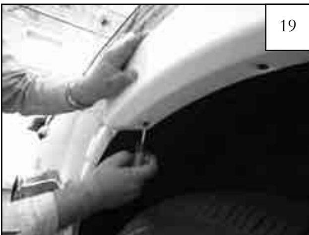
19 Start two supplied Pan Head Screws (SW1-0056) through holes in flare and into Clips (CL1-0009) installed in Step 18. Do not tighten.
