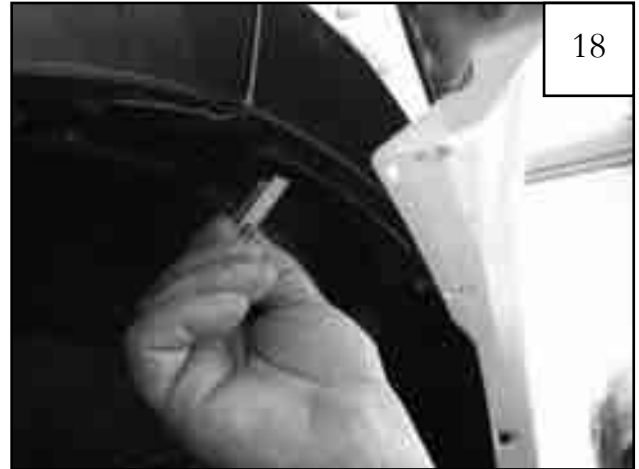
18 Pull forward portion of flare out from fender gently, and slide two supplied Clips (CL1-0009) onto fender lip, aligning holes in clips with holes in flare.
