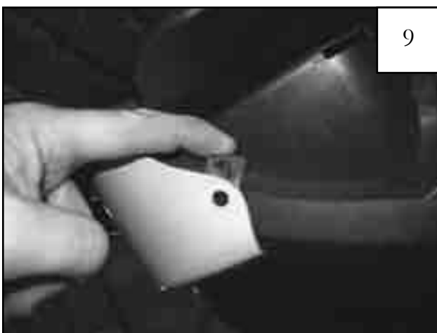
Slide an Clip/Black Tab combination (CL1-0005/MT1-0002) onto bumper lip, aligning with hole located at front underside of flare.
