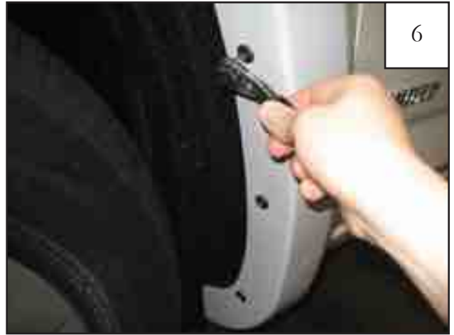
Start supplied truss-head screws through three rear holes in flare and into factory holes in rear of wheel well.
