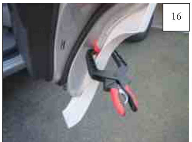
Using either a clamp or a partner, hold door piece in place so that the plastic is fully set in the clip. Starting in the two center locations, tighten screws started in step 15.
