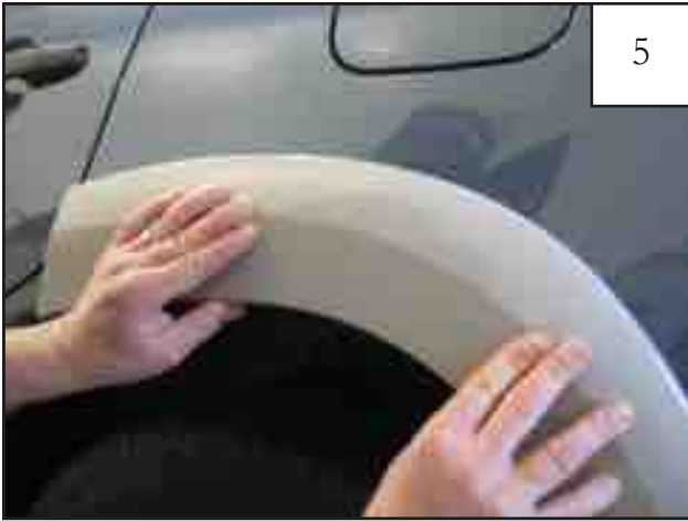
Replace flare on fender, aligning holes with holes in clips.
