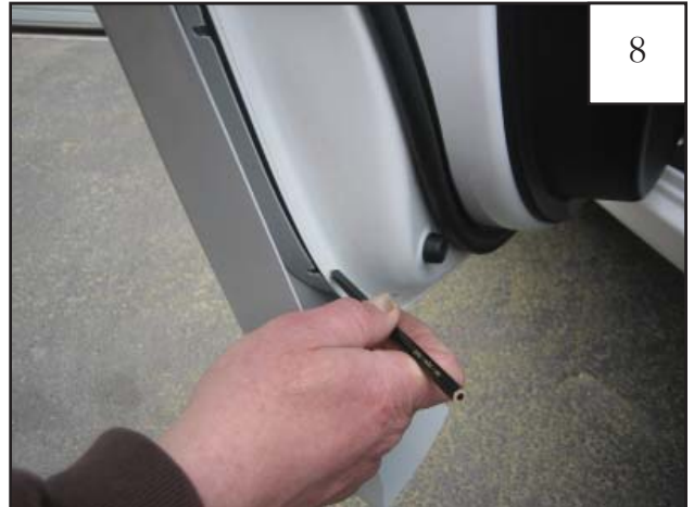
Open rear door. Make sure door piece aligns with the mark made in step 7. Using holes in door piece as a guide, mark four clip locations with a grease pencil.
