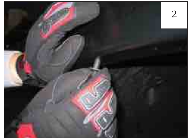
Holding flare in position on fender, install two supplied Plastic Push Retainer.
