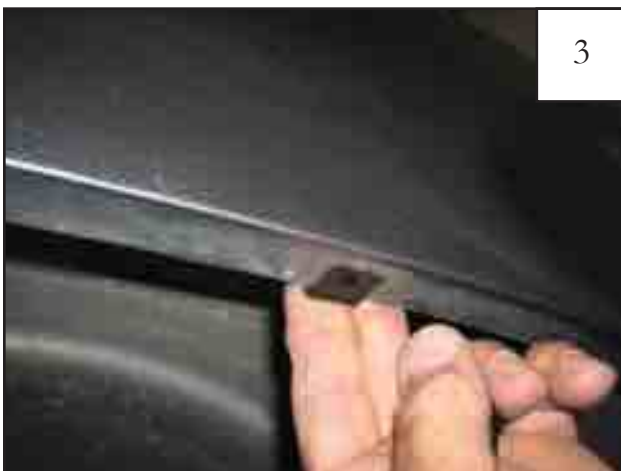
Slide a supplied Plastic Clip over two top marks made in Step 1. Clips may need to be adjusted to align with holes in flare. NOTE: the raised collar on the clip should face upward into the interior of the fender.
