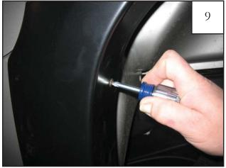
Start a supplied Serrated Flange Screw through each of the remaining holes and into each "S" Clip installed in Step 7.
