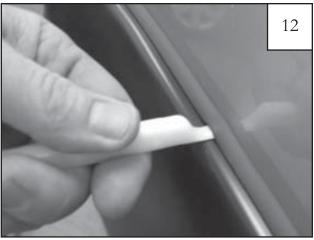
Using flat end of supplied Edge Trim Tool, seat edge trim against flare by inserting straight end between edge trim and flare at one end. Next, slide around entire edge to the other end.
