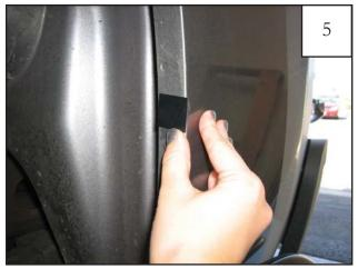
Center a supplied Black Plastic Tab over the remaining four marks made in Step 1, aligning edge of tab with inside of fender lip (tab may extend over outside of fender).
