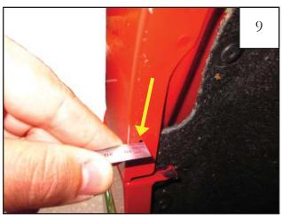
Remove the flare. At the marked locations made in Step 7, measure inward 22mm from the edge of the fender. These are the marks to be drilled.
