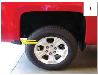
Using a T-15 Torx bit socket wrench, remove factory installed screws from factory rear mudguard. Discard screws.
