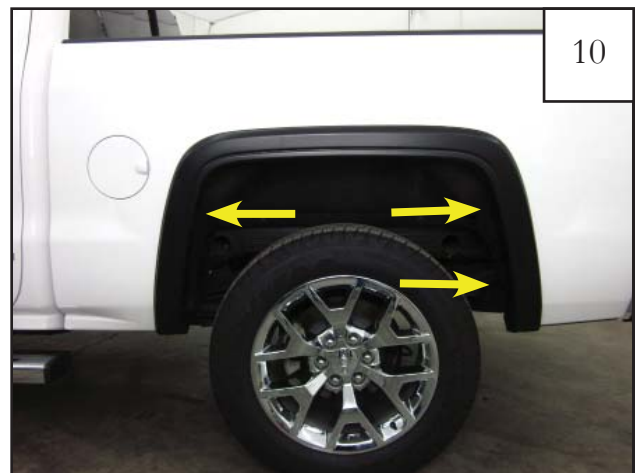
Hole locations to be marked for drilling.
