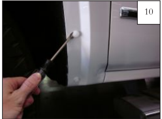
Use a pry tool to remove any remaining factory fasteners that may have stayed on the vehicle during the removal process. Clean area surface.
