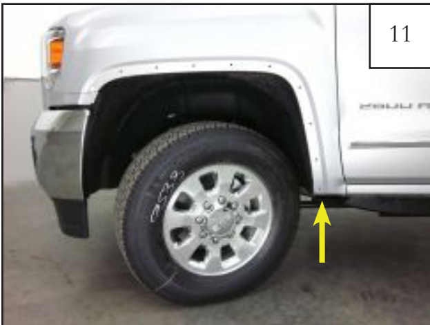
Reinstall factory fastener removed in step 8 using a 1/2" socket and wrench.
