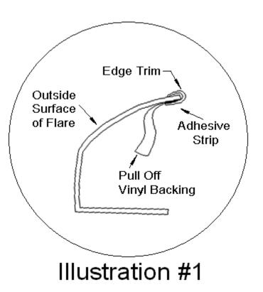
(B) Press edge trim into place along the top edge of the flare in one-foot increments, pulling red vinyl backing free as you continue to work your way around the top edge of the flare.
