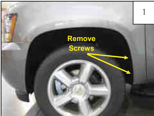
Using a 9/32" socket, remove two factory screws. Retain screws for later use.
