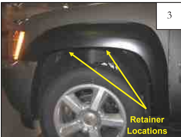
Verify fit and tightened all screws. Follow steps 1-3 for passenger side installation.
