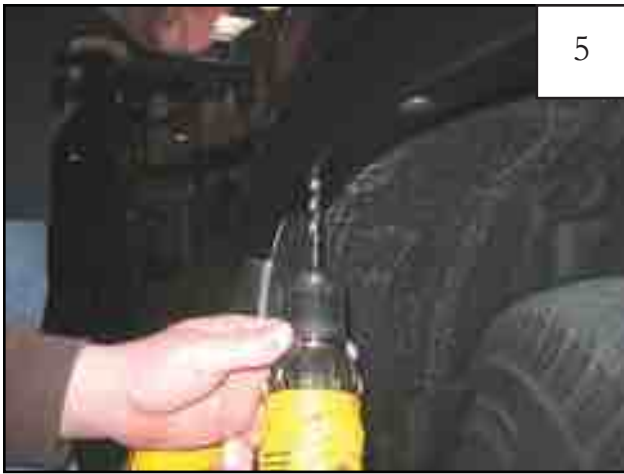
Using hole located in forward portion of flare as a guide, drill through the splash shield with a 5/16" bit. Holes in flare and splash shield should align with factory hole located in fender.
