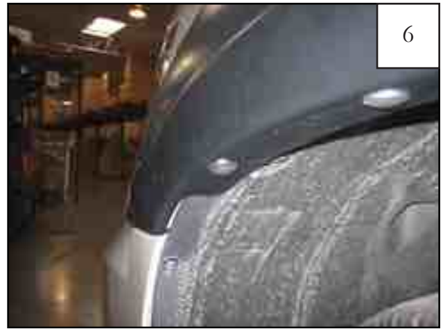
Install a supplied Retainer (RV1-P006) through hole drill in Step 5.
