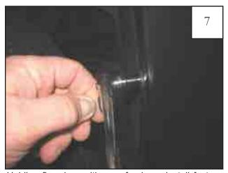
Holding flare in position on fender, reinstall factory screws removed in Step 7.
