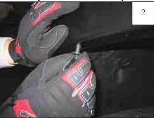
Holding flare in position on fender, install two supplied Plastic Push Retainers.
