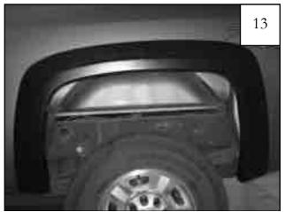
Verify fit and tighten all screws. Repeat steps 4-13 for passenger side installation.
