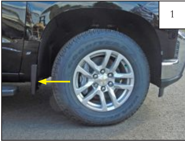
1 Locate the factory installed mud flap on the passenger side front wheel well.
