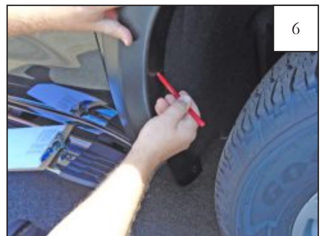
6 Use a grease pencil to mark the two locations of the holes indicated with the circles in Step 5. Remove flare from vehicle.
