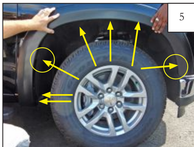
5 Hold flare to vehicle and note the approximate hole locations in the flare.
