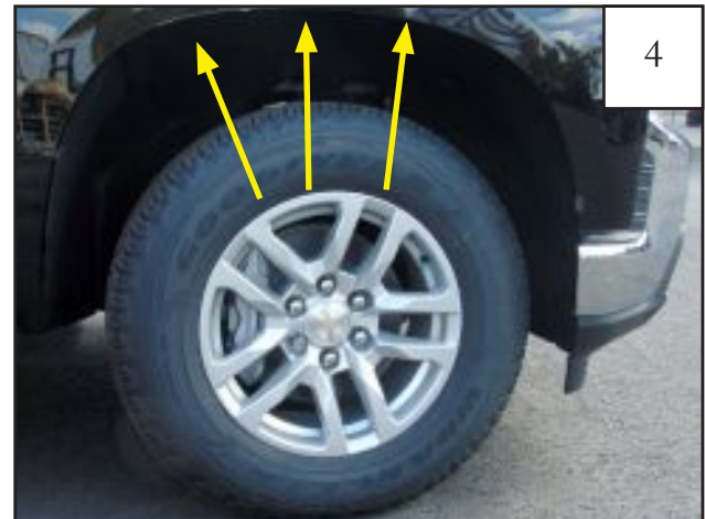
4 Remove (3) factory installed T15 screws from wheel well as shown above. These screws will be re-used to install the front flare.
