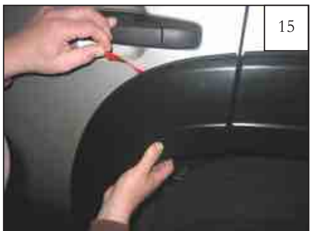
Confirm placement of the part. Gently pull the tape liner from the tape, starting with the top tab you created.
