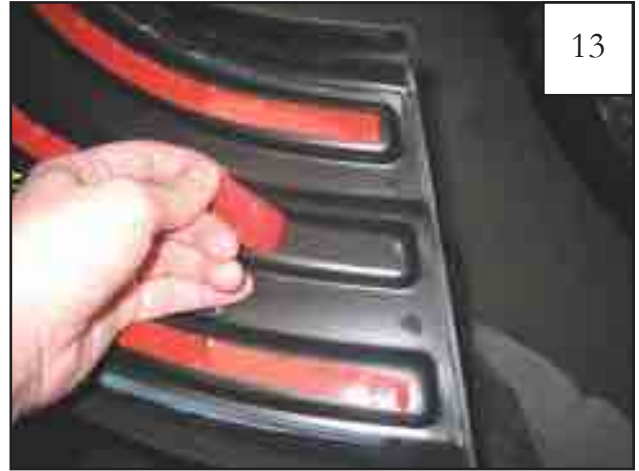
Peel the red liner entirely from the CENTER tape pad. Peel 2" of liner from each of the other two tape pads, folding out to form tabs.
