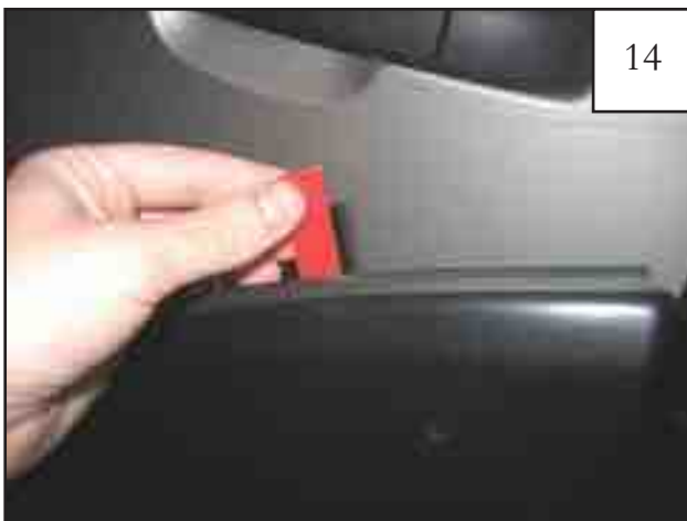
Hold the part at an angle to prevent tape from prematurely sticking, and align part on the door. Make sure liner is protruding from part for ease of removal.
