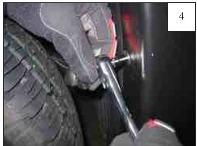
Reinstall factory screws removed in Step 1.
