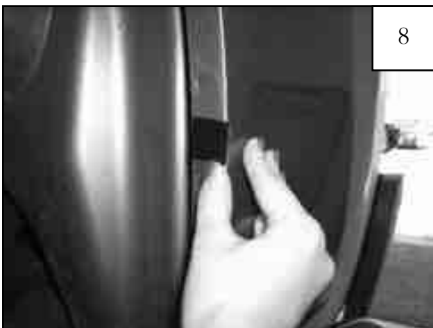
Center a supplied Black Plastic Tab over the remaining four marks made in Step 4, aligning edge of tab with inside of fender lip (tab may extend over outside of fender).
