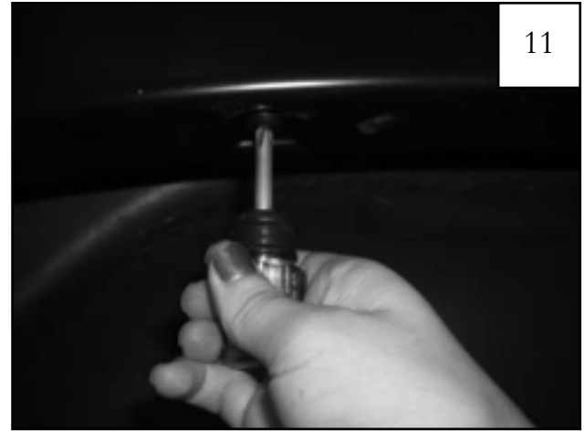
Reposition flare on fender. Start a supplied #14 Truss Head Screw through each topmost hole in the flare, and into each Plastic Clip installed in Step 6.
