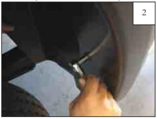
Holding flare in position on fender, reinstall screws removed in Step 1. Do not tighten. (An awl may be used to align the threaded clip with holes in flare and fender lip) *Note: Make sure screws engage in splash shield.*
