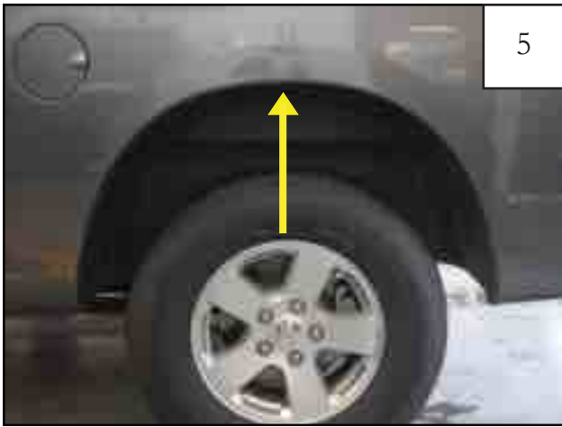
Install speed clip in this location. See steps 6-8.
