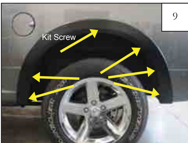
Kit supplied screw and factory installed screw locations. Install the kti supplied screw at the top of flare first for easier installation. See steps 10 & 11.
