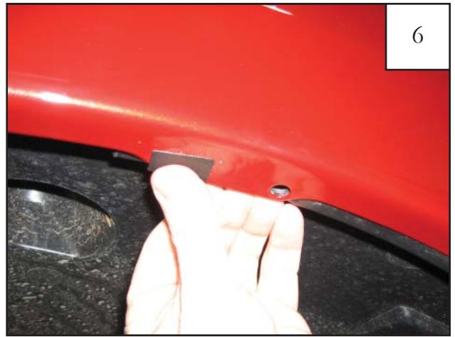
Install plastic tab over existing factory hole.
