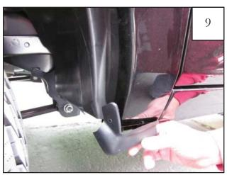
**2011 Models Only:** Remove inner piece at bottom rear of wheel well.
