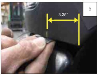
Measure 3.25" from wheel well along headlight mounting and mark with a grease pencil. Remove white backing from 1"x1.5" Black Tab. Center tab at mark, hook around lip, and install.
