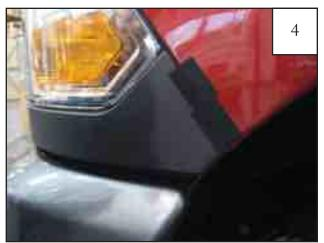
Install two 1"x1.5" Black Tabs over seam between main vehicle body and headlight mounting.
