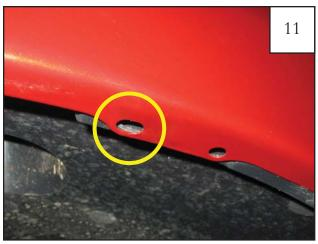
At location indicated in step 10, there is a lip with two factory holes. One hole is a circle and one is an oval. The 1"x1.5" Black Tab and #10 U-Clip will be installed over the oval. The oval is the hole more toward the front of the vehicle.
