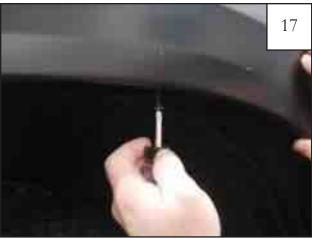
Hold flare to vehicle and start the kit supplied #8x3/4" Washer Panhead Screws with a Phillips screwdriver. *Do not tighten*.
