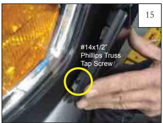
When fitting flare on vehicle, first position front piece. The #14x1/2" Phillips Truss Tap Screw hooks behind where folded 1"x1.5" Black Tab was installed in step 6.
