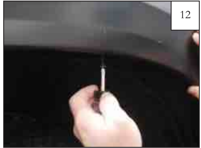
Hold flare to vehicle and start the supplied #8x3/4" Washer Panhead Screws (SW1-0056) with a Phillips screwdriver at locations show in steps 10 & 11. Do not tighten.
