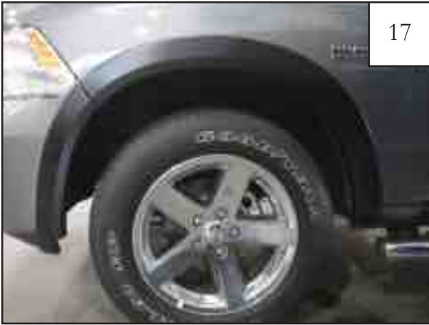
PLASTIC BUMPER ONLY: Completed front flare installation.
