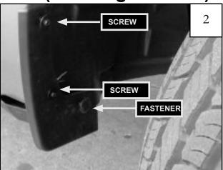
Remove (2) factory installed screws, and (1) factory installed fastener, and remove mud flap from vehicle.
