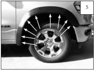
Hold flare to vehicle and start re-installing the remaining (9) factory screws with a 8mm socket. *Do not tighten*.
