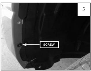
Re-install the previously removed lower factory screw as indicated above. Keep remaining screw. Fastener can be discarded.
