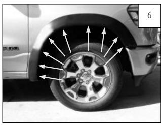
Press flare firmly against sheetmetal and tighten all screws.
