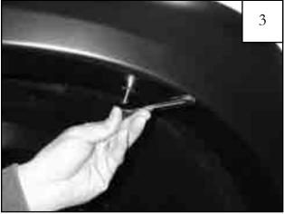
Holding flare in position on fender, reinstall screws removed in Step 2.
