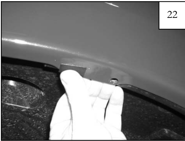
Install 1"x1.5" Black Tab (MT1-0014) over existing factory hole.
