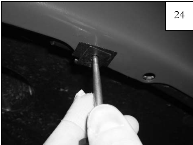
Using an awl or similar pointed tool, poke a hole through 1"x1.5" Black Tab using the #10 U-Clip hole as a guide.
