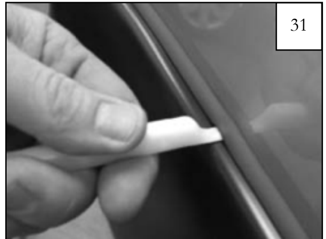
Using flat end of supplied Edge Trim Tool, seat edge trim against flare by inserting straight end between edge trim and flare at one end. Next, slide around entire edge to the other end.
