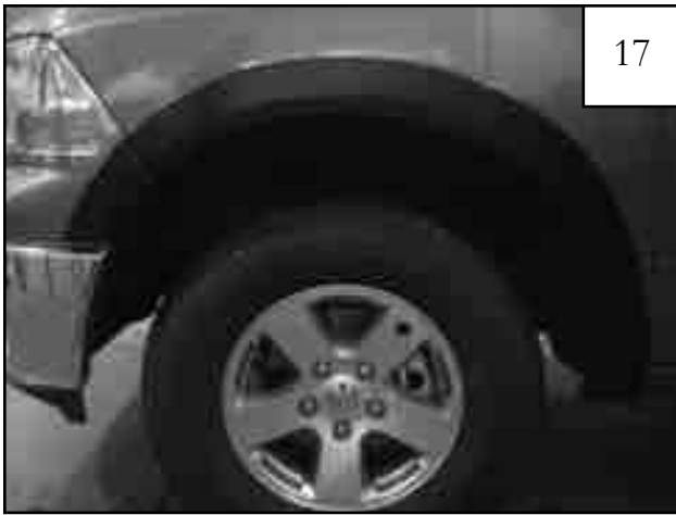
METAL BUMPER ONLY: Completed front flare installation.
