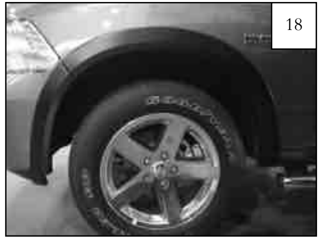
PLASTIC BUMPER ONLY: Completed front flare installation.
