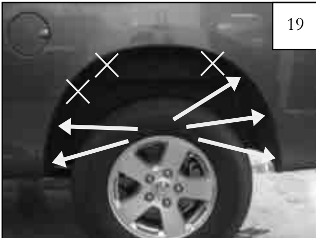
Remove these five factory installed screws using an 8mm socket wrench.
