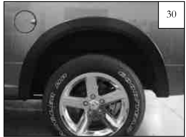
Completed rear flare installation.
