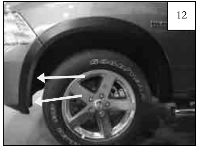
PLASTIC BUMPER ONLY: Additional supplied screw locations.
