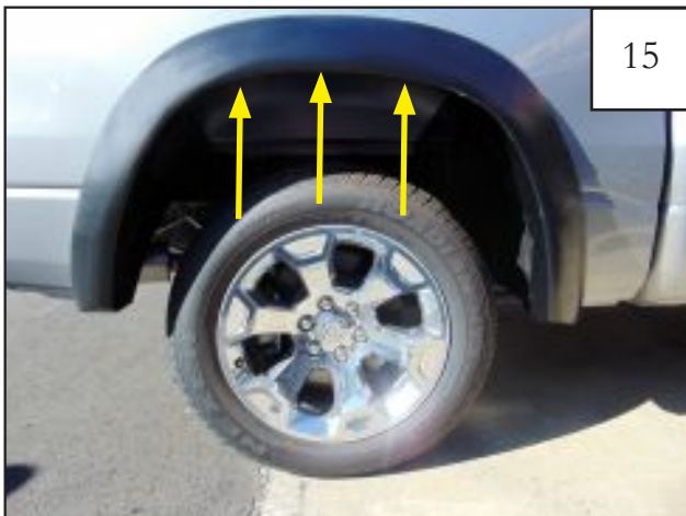
Hold flare in place and start Screw (SW1-0056) using a Phillips screwdriver in (3) locations as shown. Do not tighten. Continue to Step 18.
