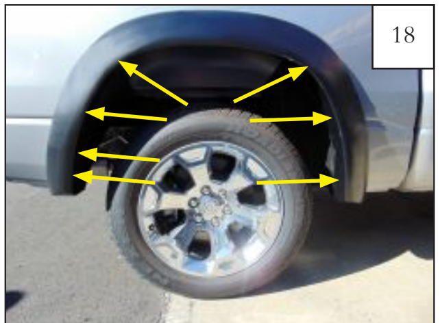
Continue holding flare in place while you start reinstalling (7) factory screws using an 8 mm socket wrench. Do not tighten.
