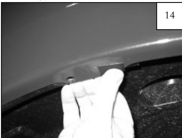
Install plastic tab over existing factory hole.
