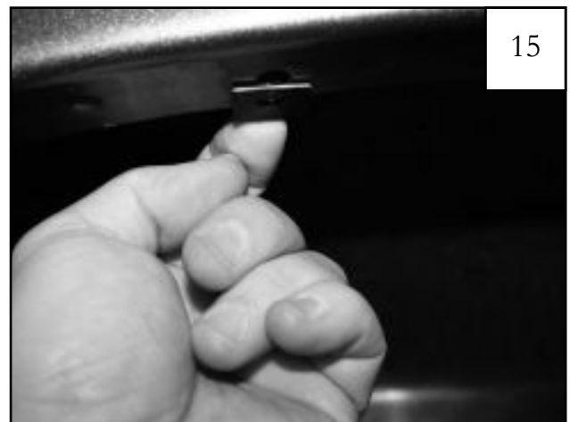
Install Clip (CL1-0022) over existing hole.
