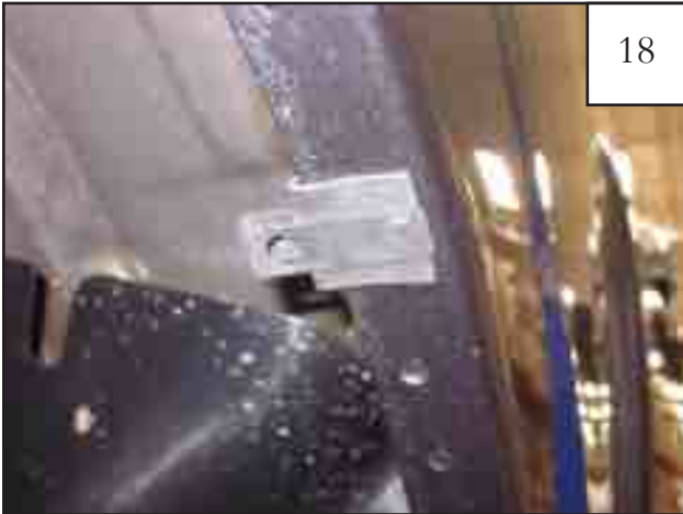
Install supplied long clips (CL1-0009) over the foam tabs.
