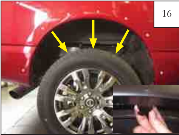
After removing the Factory flare, remove 3 factory installed clips.
