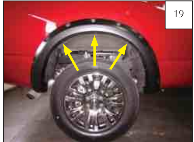
Position flare on rear fender and install 3 supplied screws (SW1-0058) through flare and into the clip holes.
