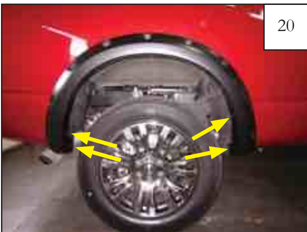
Install 4 supplied screws (SW1-0049) through holes in flare and into the existing factory holes.
