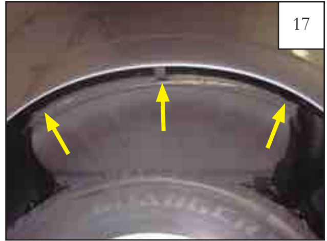
Install a foam tab (MT1-0034) over 3 top center metal tabs in the wheel well
