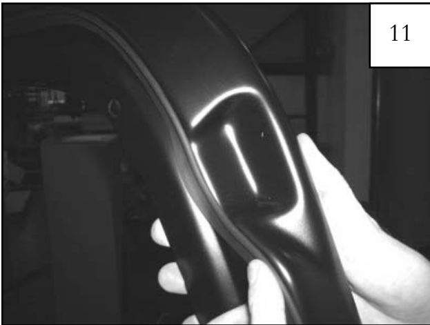
When positioning gimp around latch section for front, make sure round edge of gimp is positioned below the edge of the part (Gimp will continue over entire length of part).
