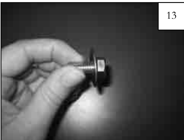
Position Inner Flare Piece on fender, aligning existing 5/16" holes in Inner Flare Piece with holes on fender. Slide a supplied 1" Fender Washer onto supplied Hex Head Bolt.
