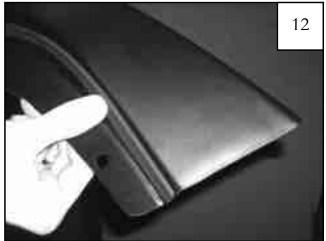
After gimp is properly placed, press to adhere properly and cut ends flush with ends of flare.
