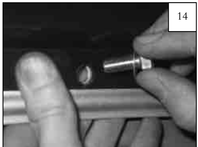
From inside of fender, hold a supplied 1" Fender Washer over hole. Insert a Bolt/Washer assembly through Inner Flare Piece, fender and washer on backside of fender.
