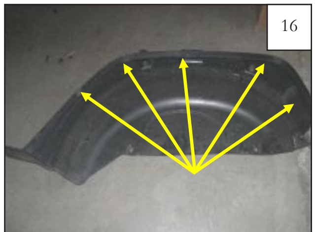
#14 U-Clip locations. NOTE: The rearmost hole will NOT have a clip.
