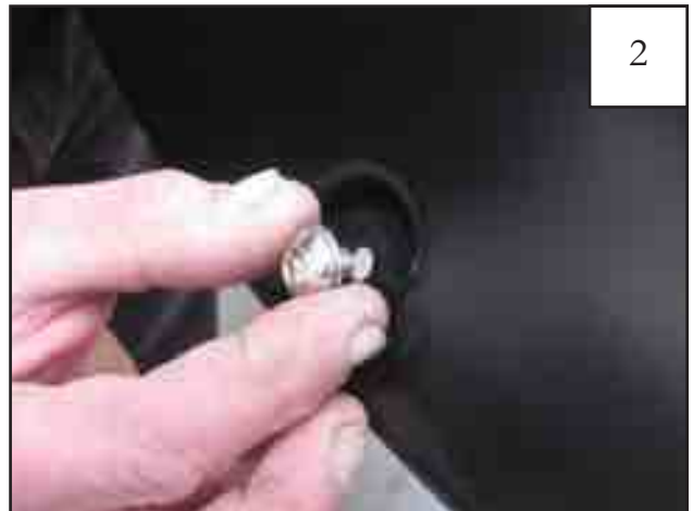
Put each Bolt/Washer combination through a pocket hole in the flare, with the Bolt head and Washer on the outside.
