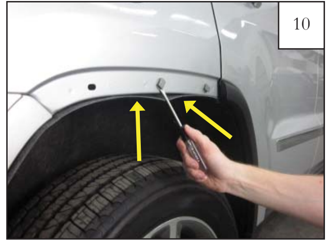
Use a pry tool to remove any remaining factory fasteners that may have stayed on the vehicle during the removal process. Remove factory fasteners from wheel well liner (2 places indicated by arrows).
