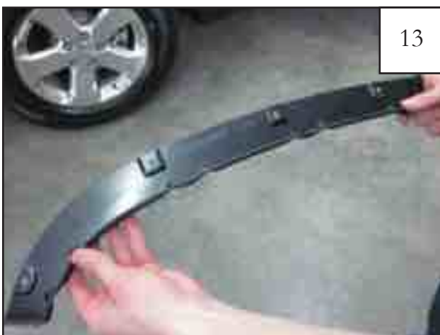
Locate the Door Flare Inner Piece. Inner Door Pieces are marked "Passenger Side" & "Driver Side".
