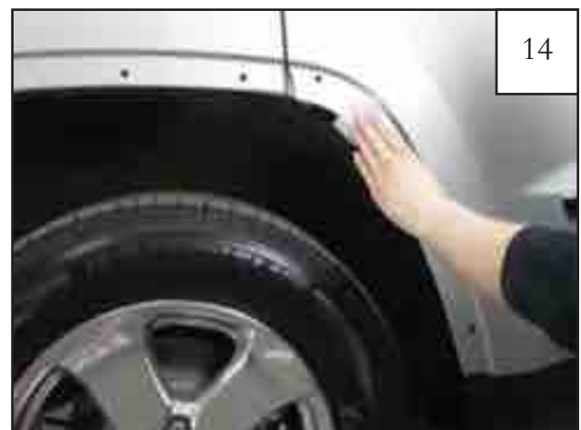
Using provided Alcohol Prep Pad (AD1-0010) wipe down area where Inner Door Piece tape will be adhered to vehicle.
