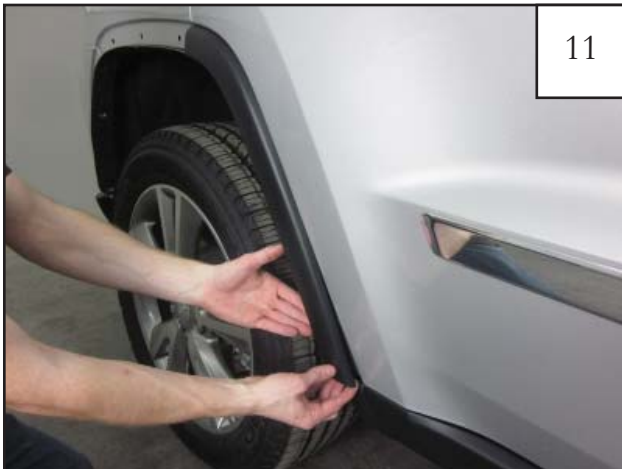
Starting at front of factory door flare, firmly grip part and pull to remove from vehicle. Note: You will hear popping sounds as the factory fasteners release from vehicle. This is normal.
