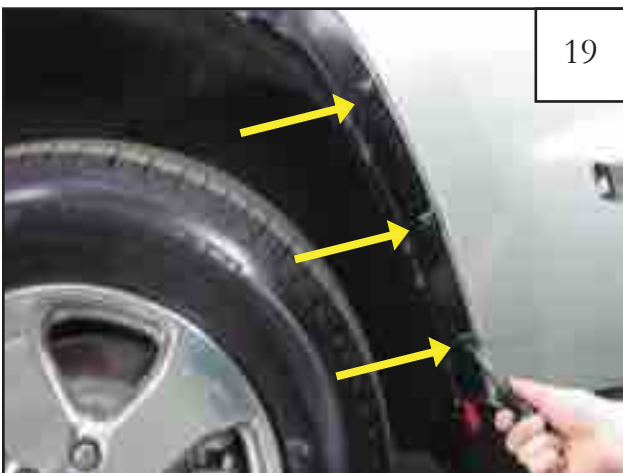
19 Use a Phillips Head Screwdriver to install provided Screws (SW1-0044) into the three remaining hole locations. Do not fully tighten at this time.
