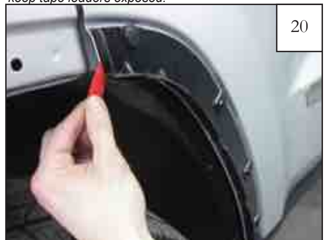
20 Remove red tape liner from inner piece.
