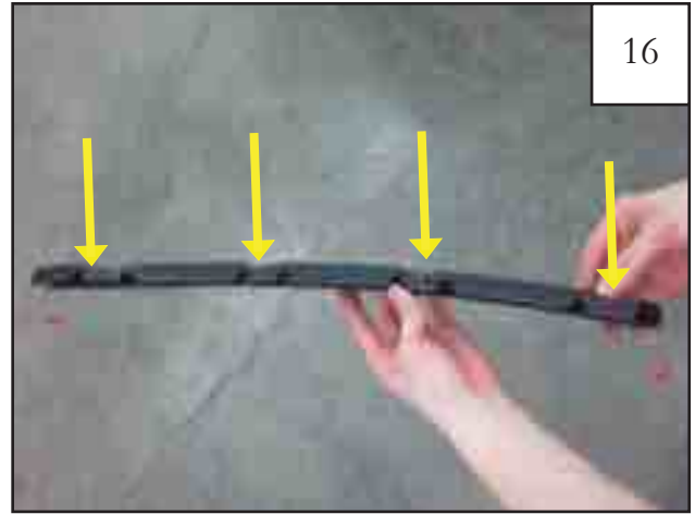
16 Inner Piece Clip (CL1-0023) locations (4 places). See next step (17) for a closer view of clip locations.
