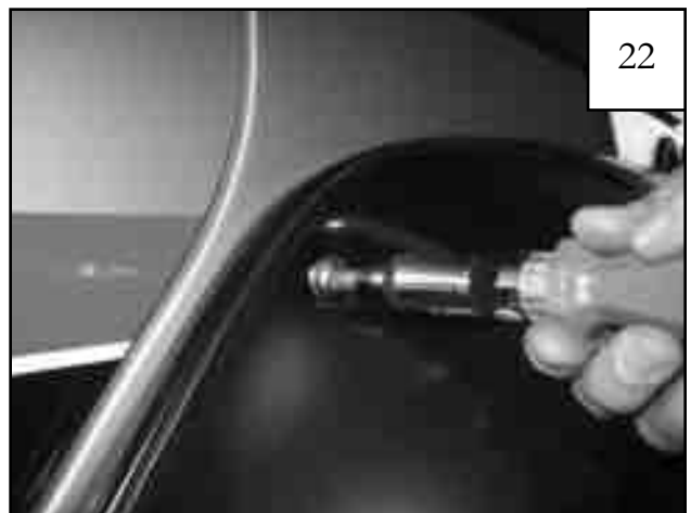
Start Screws/Washers through pocket holes in flare and into "U" Nuts installed in Step 11 (8 places) starting at the front and working your way to the back. Do not tighten.
