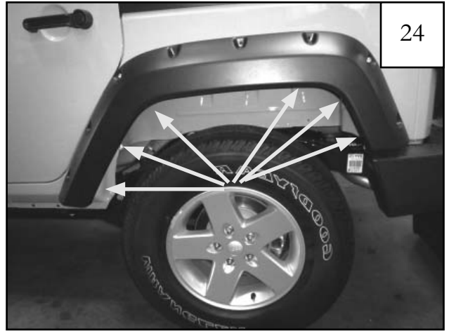
Truss Head Screw Locations.
