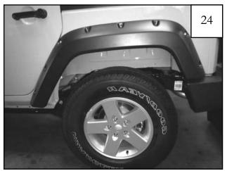
Ensure fit, and tighten all screws
