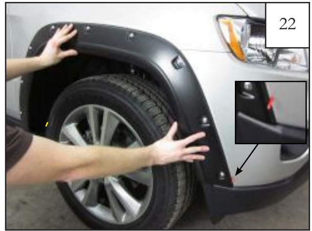
Hold the front Flare onto vehicle ensuring tape liners are exposed on both side of flare.
