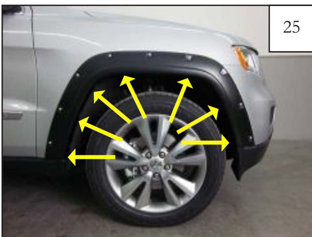
Screw/Clip locations (7 places). Ensure flare is properly aligned on vehicle and fully tighten all fasteners using a #2 Phillips Stubby Screwdriver.
