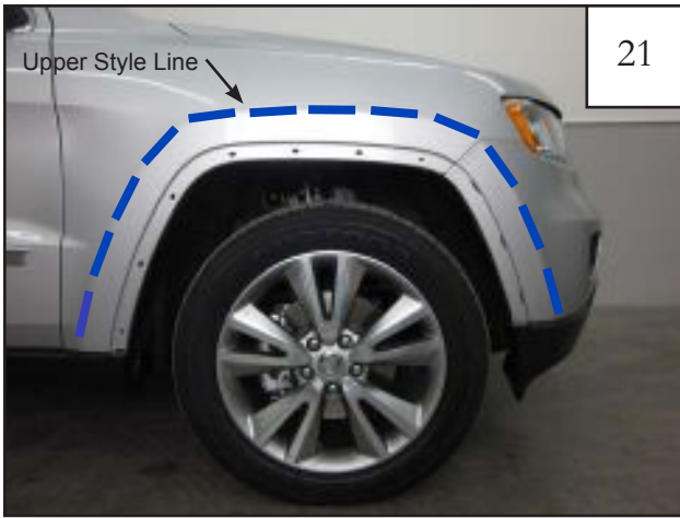
Using provided alcohol prep pad (AD1-0010), clean sheet metal of fender and bumper for front flare installation. Use upper style line on fender as a guide.
