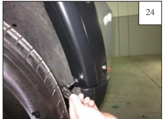
Using a Phillips head bit with a right angle screwdriver, install supplied screws (SW1-0056) thru flare and into clips installed in steps 17 & 18. Do not fully tighten at this time.
