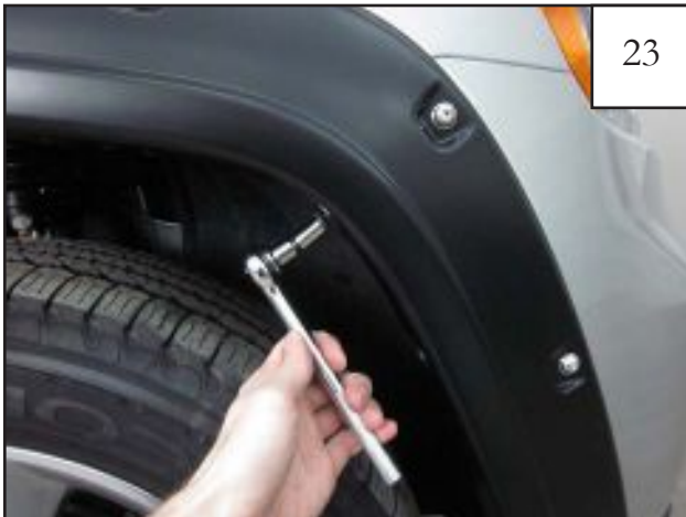
While holding Flare on vehicle, install factory fastener removed in Step 6 using a 10mm socket and wrench. Do not fully tighten at this time.
