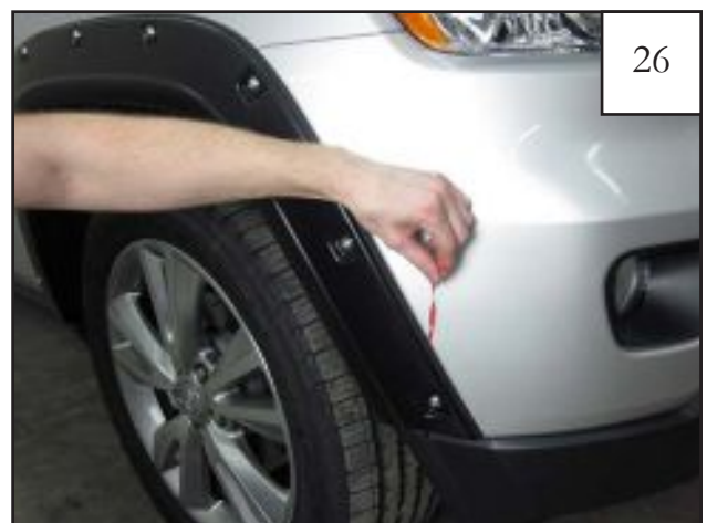
Remove the red tape liner from edge trim. Note: Be careful not to tear red tape liner during the removal process.
