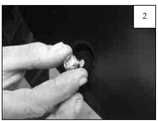
Put each Bolt/Washer combination through a pocket hole in the flare, Bolt head and Washer on the outside.
