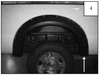
Using a 10mm socket, remove factory hex bolt located at lower front wheel well. Save screws for reinstallation.
