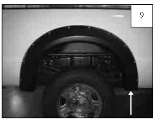
Place flare on fender and reinstall bolt removed in Step 4.
