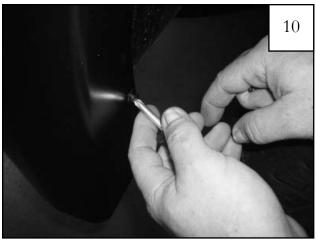
Install four supplied Screws (SW1-0050) through remaining holes and into clips installed in Step 8, working from front to back of wheel well.
