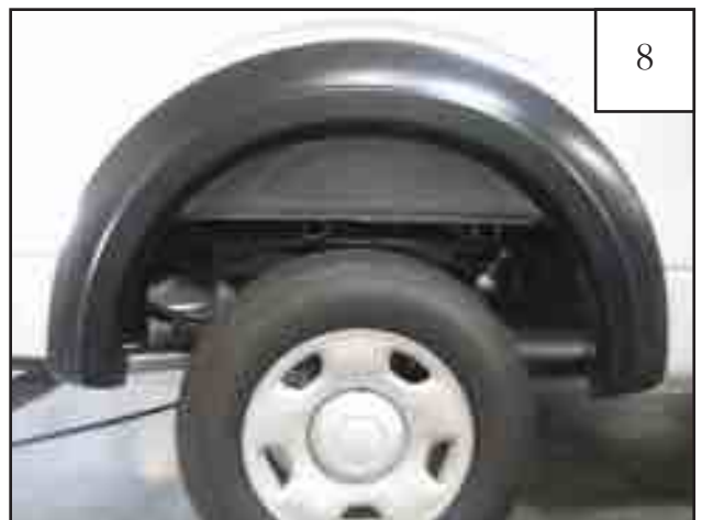
8 Completed rear flare installation.
