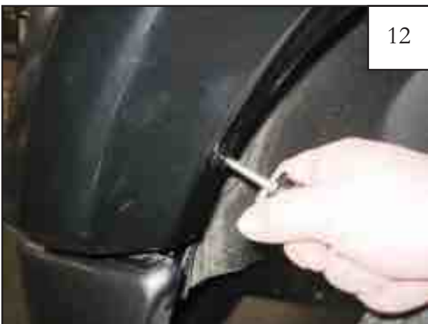
Still holding flare to fender, install Retainers (RV1-P001) using a Phillips screw driver. See Step 13.
