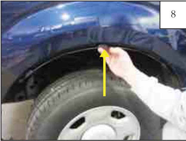
Using a Phillips screw driver, start a factory supplied screw through center hole in inner piece and through the Clip (CL1-0011) over the fender wheel well lip.
