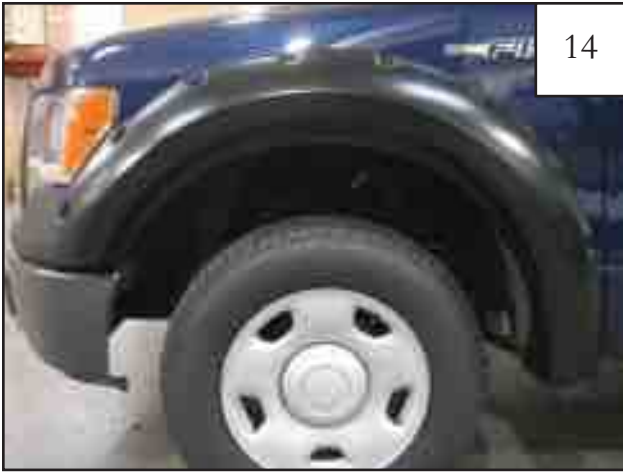
Completed front flare installation.
