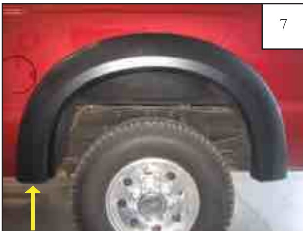
Reinstall bolt removed in Step 1 with a 10 mm socket.
