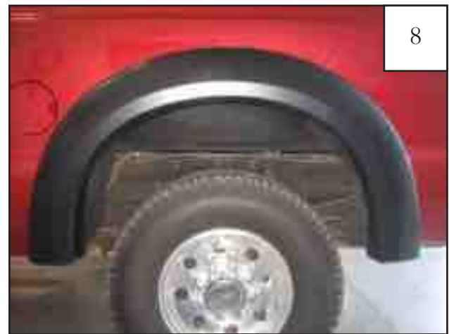
Completed rear flare installation.
