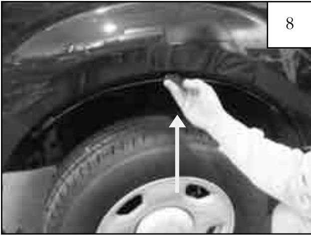
Using a Phillips screw driver, start a factory supplied screw through center hole in inner piece and through the speed clip over the fender wheel well lip.
