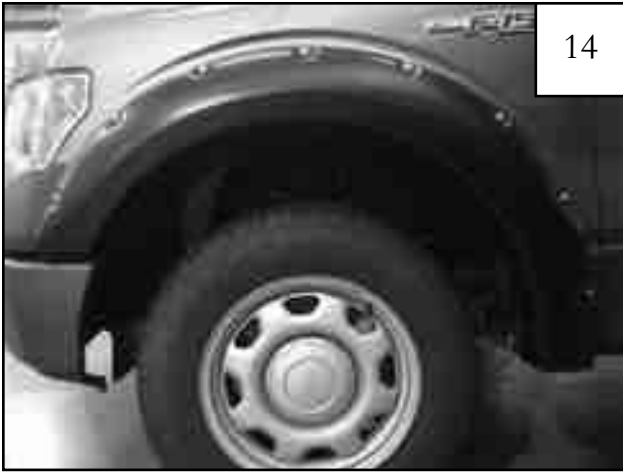
Completed front flare installation.
