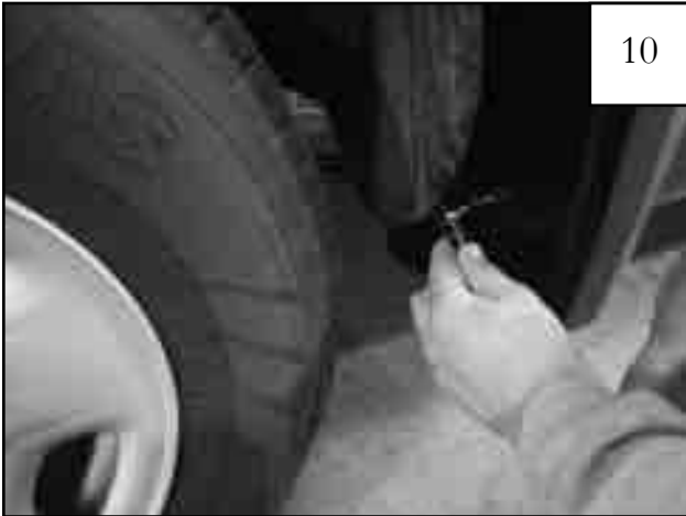
Position and hold flare on fender and reinstall rear most factory screw using a 7/32" socket wrench.
